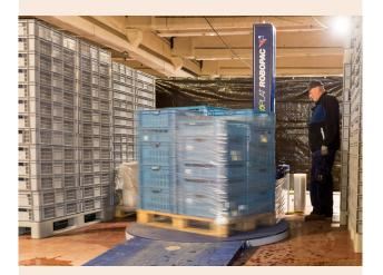
A wrapper to wind loaded pallets with plastic.
